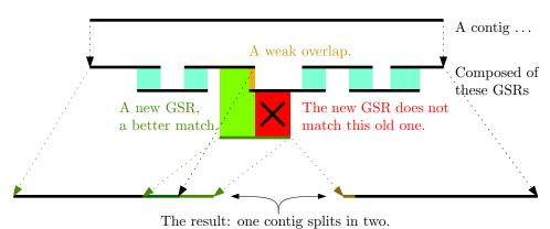
(b) If two of the GSRs in a contig have a sub-optimal overlap, they may be assembled incorrectly (yellow). If the correct GSR is found (green), it will out-compete the sub-optimal overlap and displace the bad GSR (red). The result is the split of the original incorrectly assembled contig into two smaller contigs.
